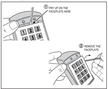
Figure 6. Removing the Faceplate
